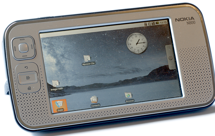
Figure 2.2: Nokia N800 running NITdroid (Android port)
